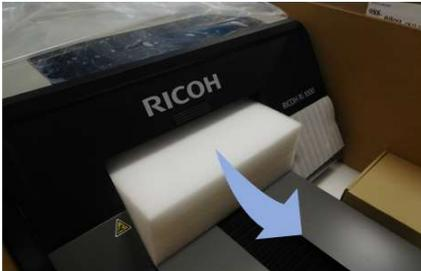
Table in printer is secured by Foam block. Please remove before startup
