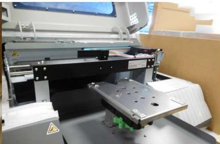
Hold foam block on the side and gently pull forward. With block removed, continue with set up steps as described in the **user manual**.
