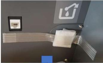
Slide drain tube through cap until it meets with the zip-tie
